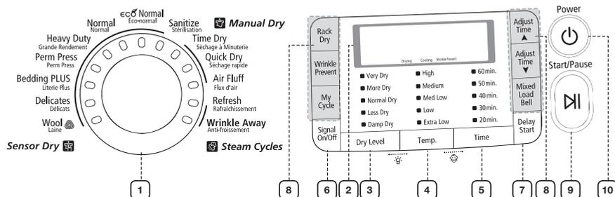
To select a cycle, rotate the Cycle Selector dial to the desired cycle. The indicator light by the cycle name will illuminate. The Normal, Heavy Duty, Towels, Perm Press and Delicates cycles are Sensor Dry cycles. Sensor Dry automatically senses the moisture in the load and shuts the dryer off when the selected dryness level (very dry to damp dry) is reached.
