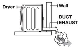
2. Use 4" diameter rigid metal duct. Tape all joints, including at the dryer. Never use lint-trapping screws.
