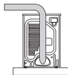
4. Clean all old ducts before installing your new dryer. Be sure the vent flap opens and closes freely. Inspect and clean the exhaust system annually.
