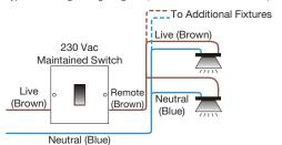
Typical Wiring Diagram (with the CLCI-1SW2EX-W)
