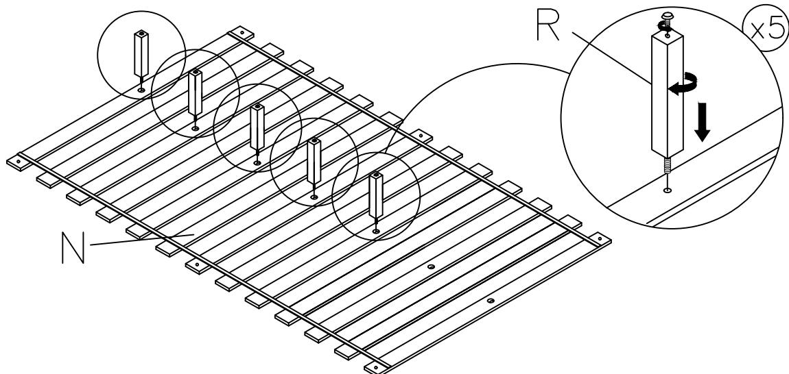
Turn Adjustable Leveler on the bottom of the Cross-Slat Support Leg leaving 6mm space between leveler and the floor.
