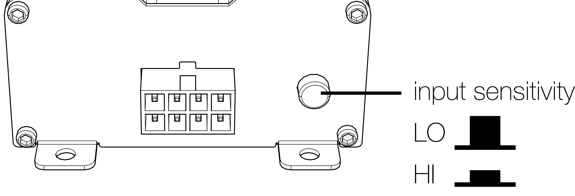
In the LO setting range, there is a  $60\Omega$  load applied for use with newer smart radios that shut off their outputs if they do not detect a speaker connected to the source unit. If there is a need to load a source unit that has an output voltage greater than 10V, please use the KISLOAD products instead of the KEYLOC's built in load resistors.
