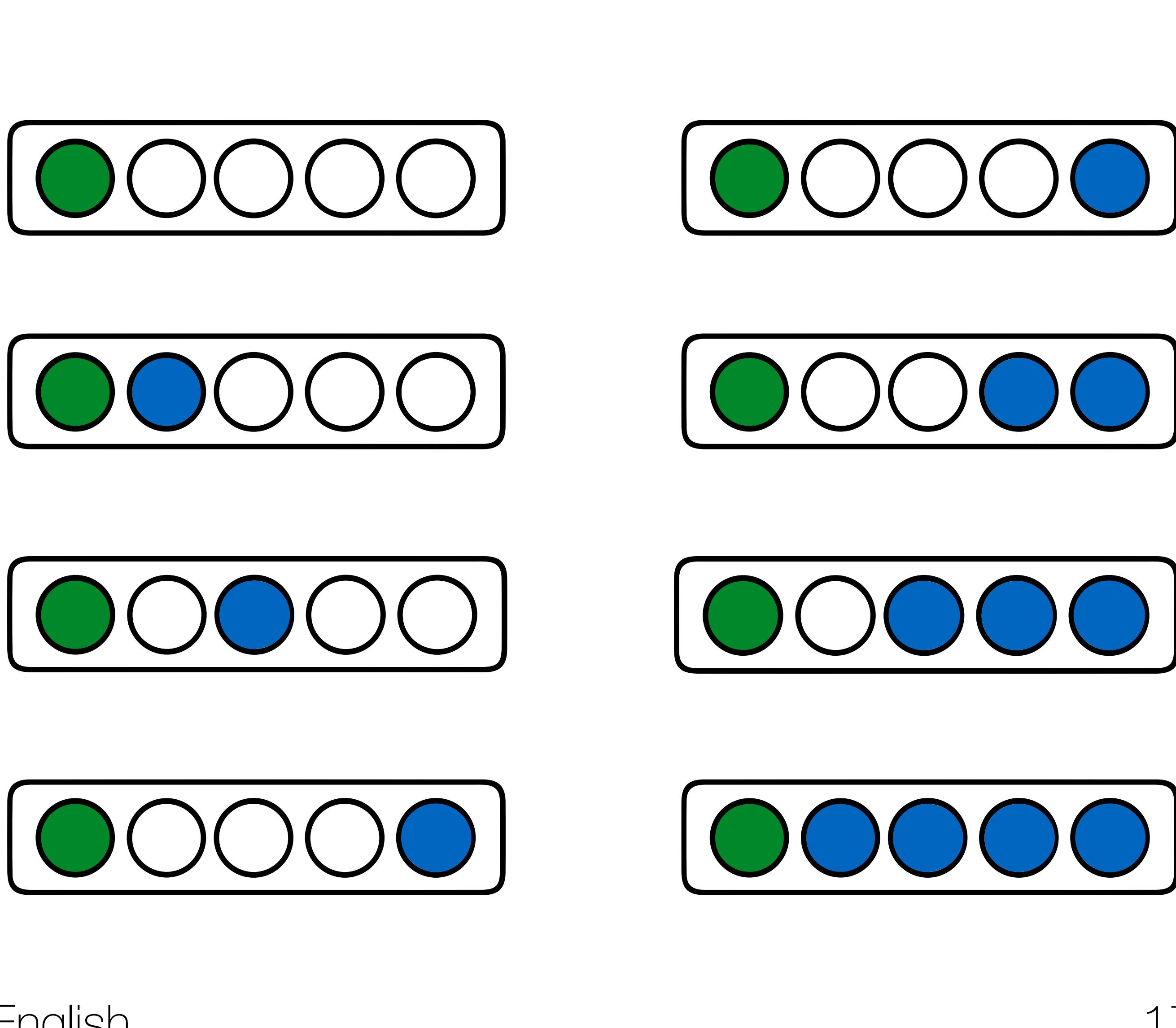
**5.** Release the KEY button. LED 1 will illuminate; LED 2-4 will turn off. You are now in the KEYLOC's Gain match mode.
