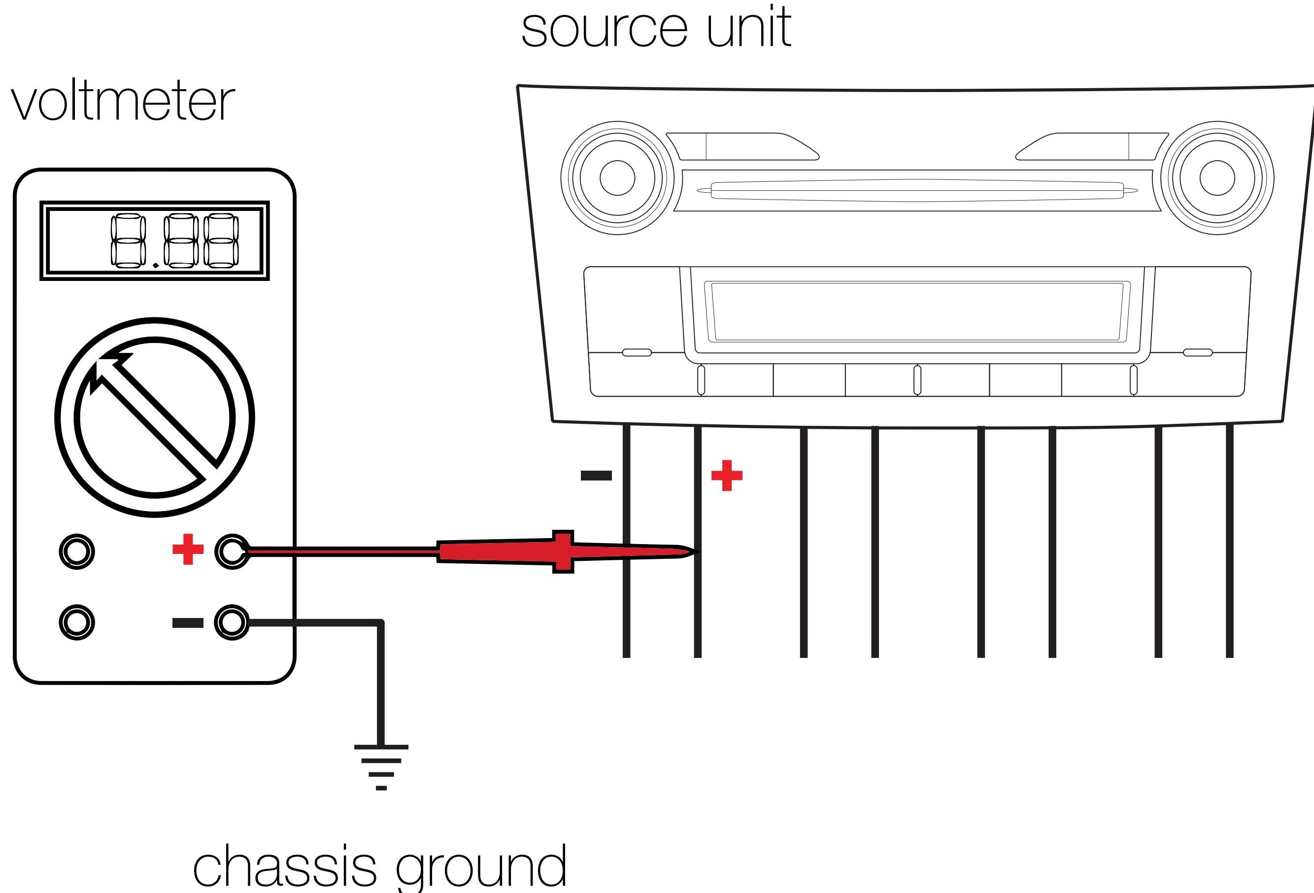
There should be a DC voltage present on your speaker lead. The DC Voltage must be between 2.5 and 6V DC to be able to turn the KEYLOC on. If it is the red Remote Turn-On wire does not need to be used. The KEYLOC will sense this DC offset to turn on, and output +12V on its remote output (up to 100mA) to turn on your aftermarket amplifier(s).
