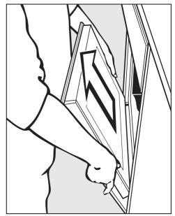
Hold the door on either side and pull it diagonally upwards from the hinge guides. Make sure that you lift the door off straight.
