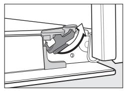
Release the locking clamps by turning them as far as they will go. Do not pull the door horizontally off its retainers, as they will spring back against the oven.
