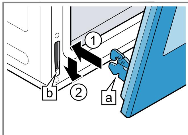
The angle of the door may need to be adjusted slightly to allow the hinges to engage properly and the door to be lowered into place. The door should lower about 3/4" (2 cm) and stop. If it does not, the hinges have not engaged properly and the door could fall if it is released.
