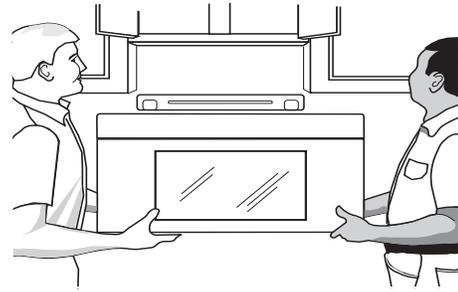
4. Using 2 or more people, lift microwave oven and hang it on support tabs at the bottom of mounting plate.
