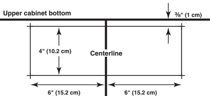
8. Mark the centerline  $\frac{3}{8}$ " (1 cm) down from the bottom edge of the upper cabinet.
