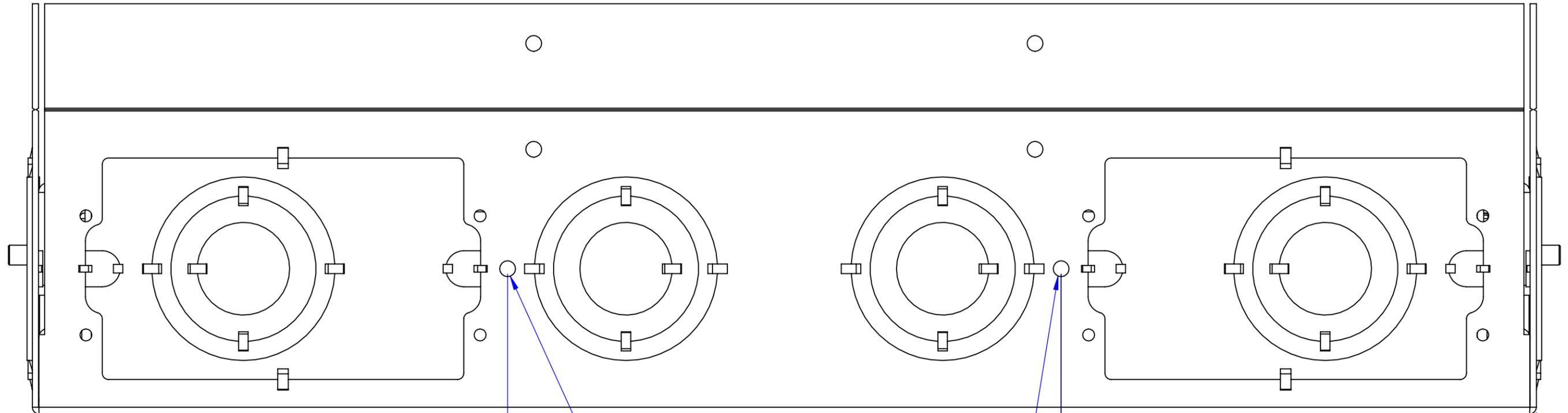
DRILL 3/16" HOLE FOR THREADFORM SCREW
