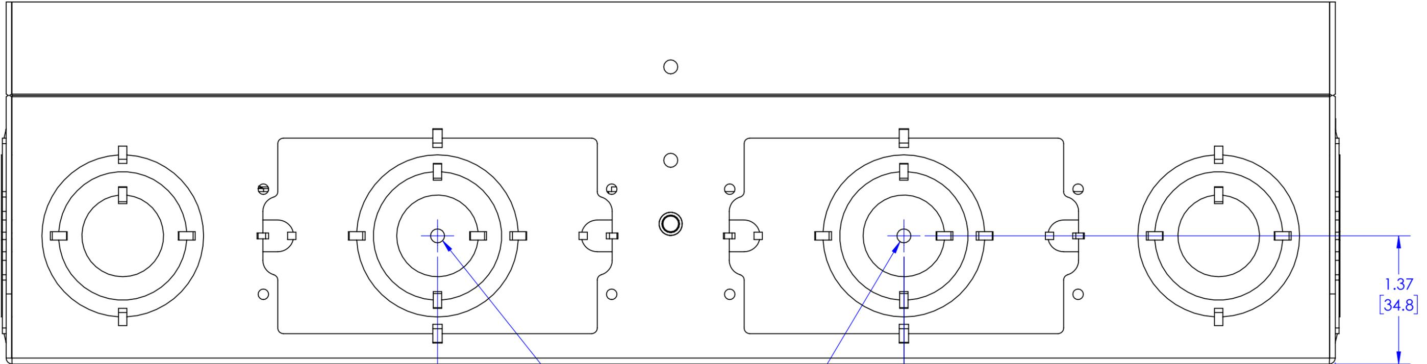
DRILL 3/16" HOLE FOR THREADFORM SCREW
