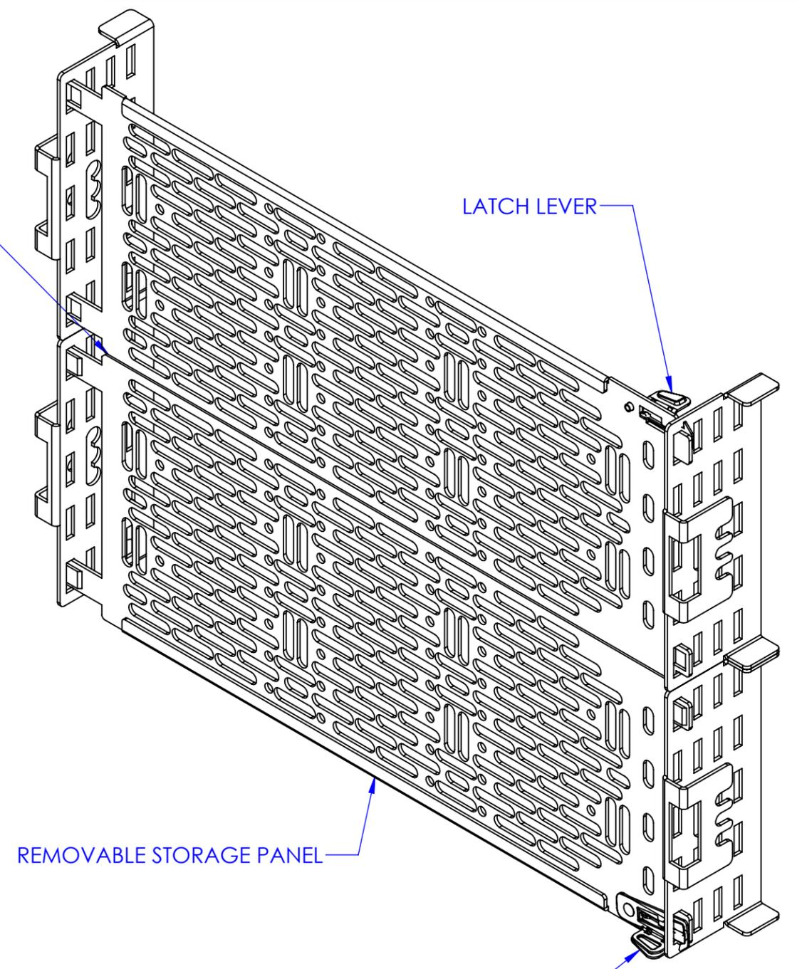
HOLES FOR ALTERNATE MOUNTING ORIENTATION
