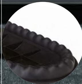
**Pleated LCS™ Linear Corrugated Surround features Ultra-Long-Travel Suspension.** The over-molded design produces truly exceptional peak-to-peak cone movement producing higher output and lower distortion—every bass note sounds distinct. Cone ribbing increases stiffness, reducing resonances to inaudible levels.
