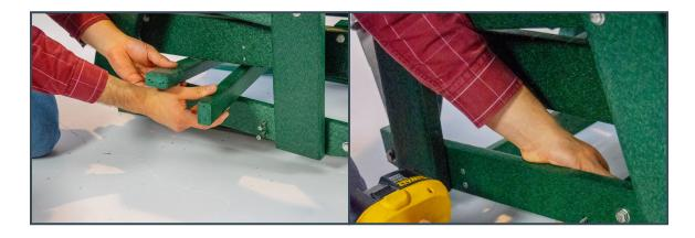
Horizontally align the front sliding brace with the screws in the bottom arm brace. Ensure the sliding brace is flush with the bottom arm brace and drive screws in. *(Repeat this process for the opposite side)*
