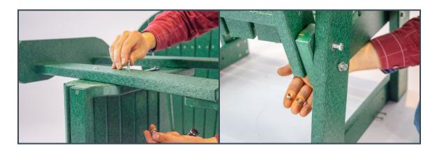
Set the seat on its side then set the arms on the side of the side ensuring the bolt holes align. Insert a short bolt into the washer, top hole of the front arm brace and seat. Slide on another washer and tighten nut onto bolt. Using another of the same bolt, repeat this process for the lower hole.
