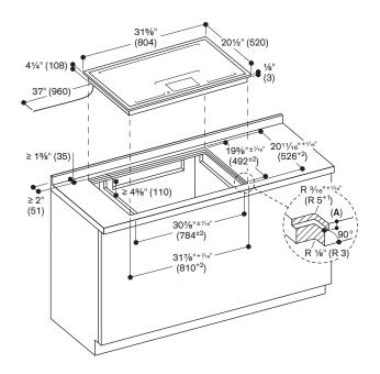
Minimum countertop thickness  $1^{3\!/_{16} \prime\prime}$  (30 mm) for flush installation.
