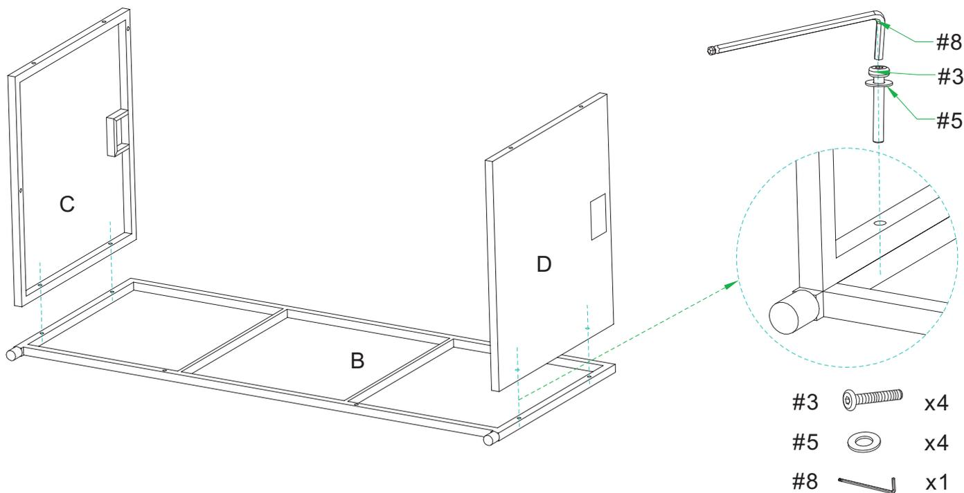
**Step2.** Attach bottom panel (part E) to left panel (part D), right panel (part C) and front panel (part B) using long bolts (part #3), flat washers (part #5) and allen key (part #8).
