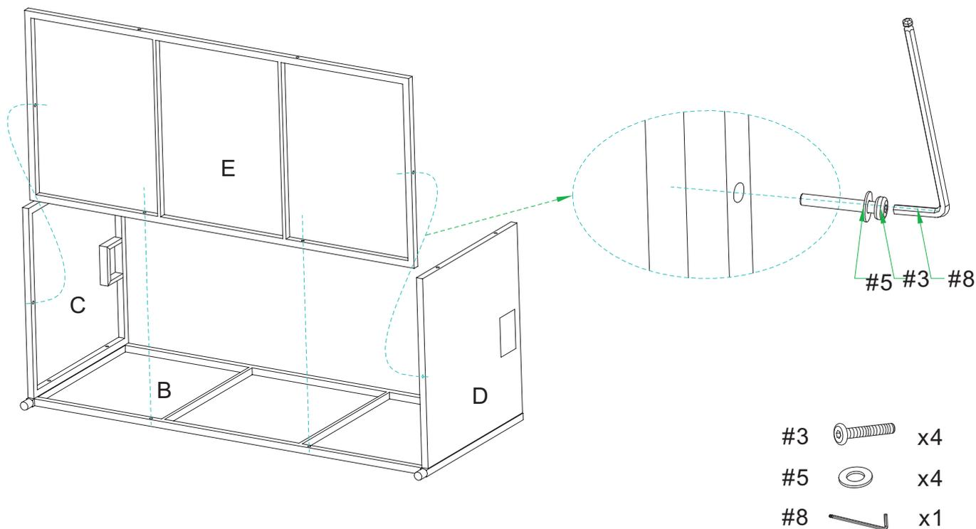
**Step 3.** Attach back panel (part A) to right panel (part C), left panel (part D) and bottom panel (part E) using long bolts (part #3), flat washers (part #5) and allen key (part #8).
