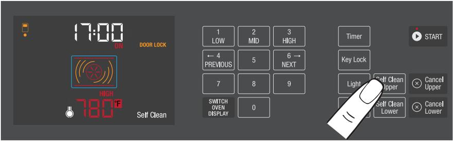
3. Select 1-Low, 2-Mid, or 3-High on the numeric keypad to set desired cleaning level.
