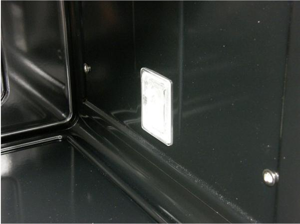
3. Using a screwdriver, gently pry protective glass cover away from oven side wall and remove from oven side wall.
