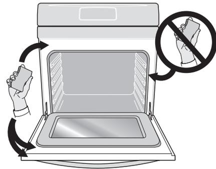
Figure 20: Clean around the oven door gasket
