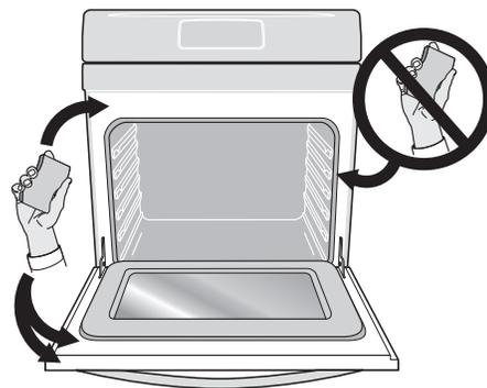
Figure 21: Clean around the oven door gasket
