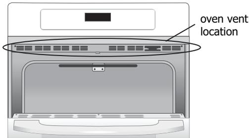
Figure 1: Do not block oven vent location
