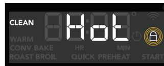
5. Once the oven has cooled down (about 1 hour) and **Hot** is no longer displayed, the oven door may be opened.
