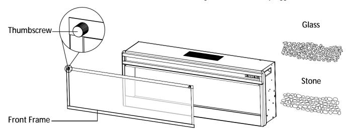
Thumbscrews are attached on front frame and are meant to be permanent and should not be removed.
