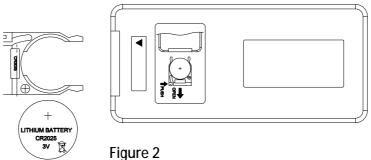
3. Insert the battery with the button side into the battery bracket, making sure the battery is firmly seated. (figure 3)
