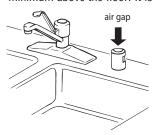
drain hose either be looped up and securely fastened to the underside of the counter or be connected to an air gap.
