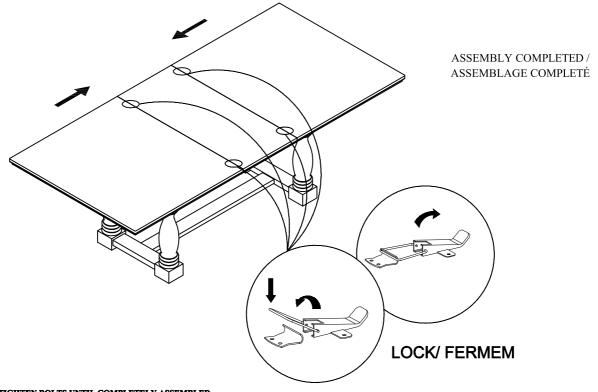
DO NOT TIGHTEN BOLTS UNTIL COMPLETELY ASSEMBLED. NE PAS SERRER LES BOULONS JUSQU'À CE QUE LE MONTAGE SOIT COMPLETMENT TERMINE MADE IN VIETNAM / FABRIQUÉ AU VIETNAM
