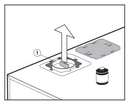
■ Pull the red transit restraint ① up and out using, e.g., universal pliers.
