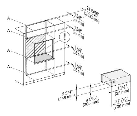
A Cutout (min. 28 sq in/ 18,000 mm<sup>2</sup>) for power cord, water hoses, and ventilation
