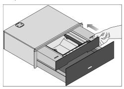
Place a thumb in front of one of the protrusions on the side of the vacuum-sealing compartment. Place your remaining fingers on the side of the vacuum-sealing compartment.
