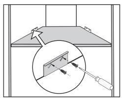
■ Secure the anti-tipping mechanism to the right and left-hand side walls of the housing unit with the 4 screws supplied 3/16" x 5/8" (4 x 16 mm).
