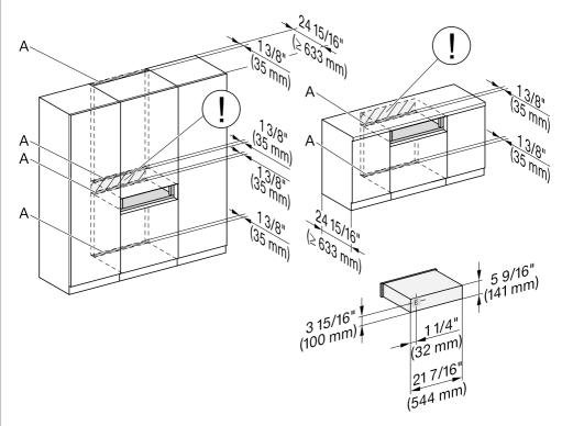
A Cutout (min. 28 sq in/18,000 mm<sup>2</sup>) for power cord, water hoses, and ventilation
