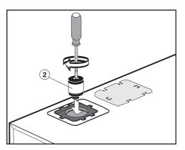
Screw the air filter ② onto the vacuum pump using a screwdriver.
