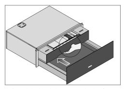
Reach behind the recess in the front of the vacuum-sealing compartment from below and push the vacuumsealing compartment back completely.
