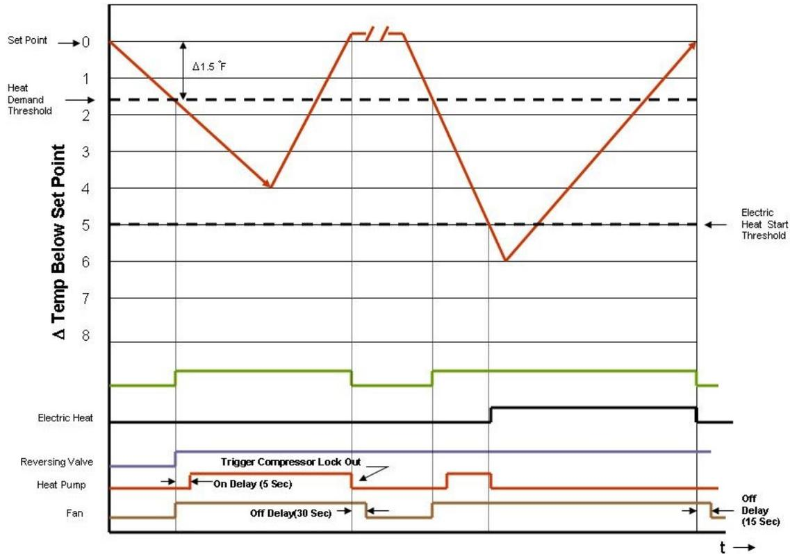
Figure 344 Heat Control (Heat Pump & Electric Heat)
