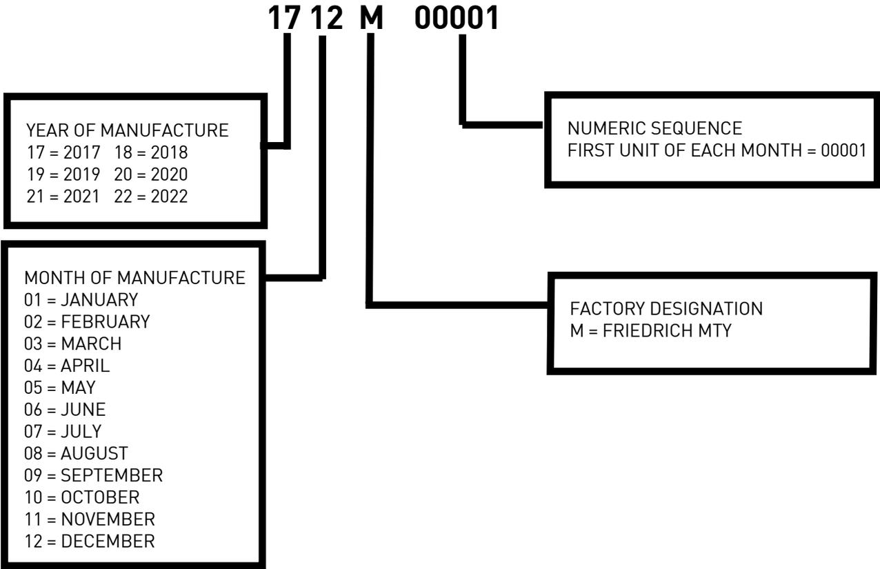
Figure 105 (Serial Number Reference Guide)
