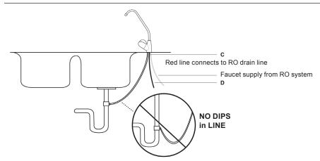
as possible and that there are no dips, loops, low spots or kinks. (See D in Figure 2 above). Also, to reduce noise, assure that RO drain line enters the vertical pipe from a direction other than the direction of entry of the garbage disposal pipe.
