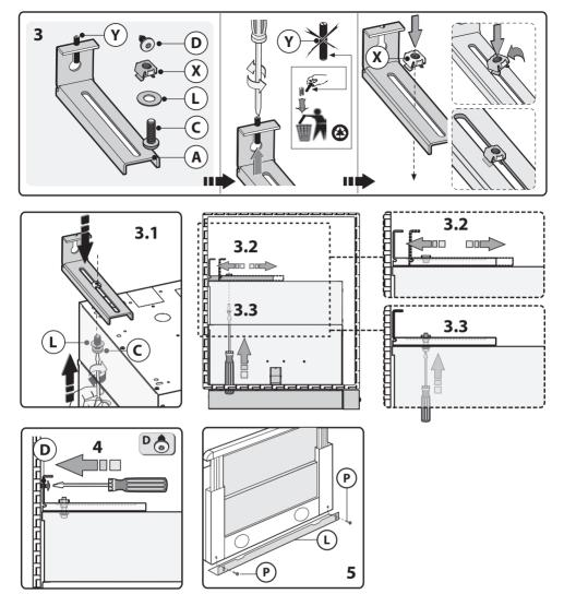
firmly reaches the wall unit (figure 4 - step 3.2). After any adjusting, tighten the bracket to the body (figure 4 - step 3.3).
