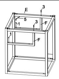
Step 3: Attach Shelf Frame (F) to LSF Leg Frame (B) and Table Base Rail (E) using Small Bolt (1) and Long Bolt (3) as shown. Tigthen with an Allen Key (5).
