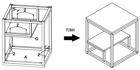
Step 4: Place Table Top (A) on a soft and clean surface to prevent finish from scratching. Place the table assembly in Step 3 onto Table Top (A). Insert Medium Bolt (2) into the holes of Table Top Side Rail (D) and LSF/RSF Leg Frame (B,C), and secure with an Allen Key (5).
