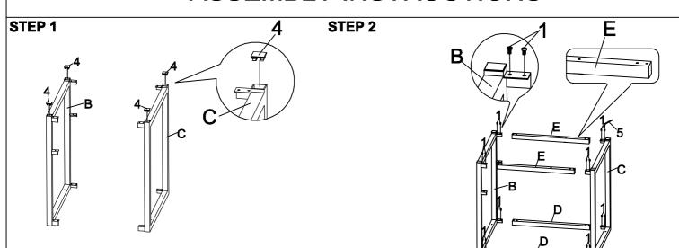
Step 1: Insert Cap (4) into LSF/RSF Leg Frame (B,C) as shown.
