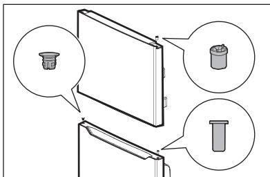
7. Remove the refrigerator door stopper and install it on the other side of the door. Remove the freezer door self-locking block and stopper. Save them to reuse. Take out the left self-locking block and stopper from the accessory
