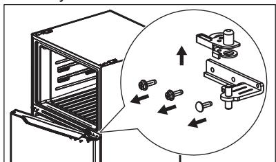
4. Unscrew and remove the bottom hinge.
