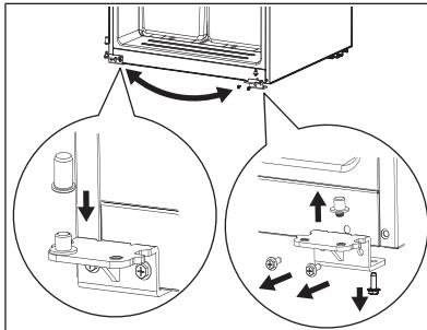
6. Dismantle the sleeves from the top right of doors and hole cap from top left of doors, and assemble them on the other side.
