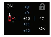
The padlock will instead be closed if the user has activated some functions (described in paragraph "6.1. Functions" on page 17); in this situation, the user will no longer be able to change the temperatures of the compartments until the function is completed or if it is disabled manually.
