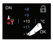
2) Scroll the values up or down to select the desired temperature (in the case of the Cantina compartment, the temperature can be set from +4°C (39.2°F) to +18°C (64.4°F)
