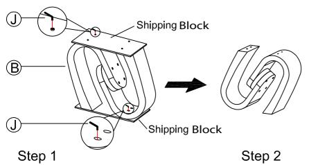
Remove the upper and lower shipping block from the pedestal
