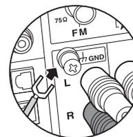
If the turntable has a ground wire, connect it to the GND terminal.
