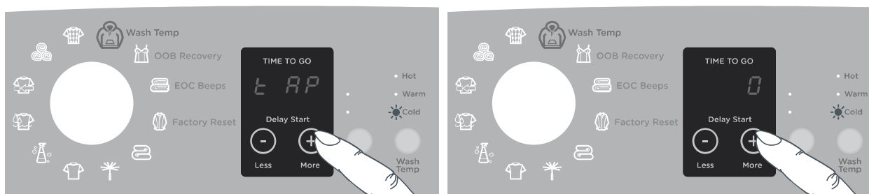
Fig.26 Changing the Cold wash temperature setting to Controlled Cold
