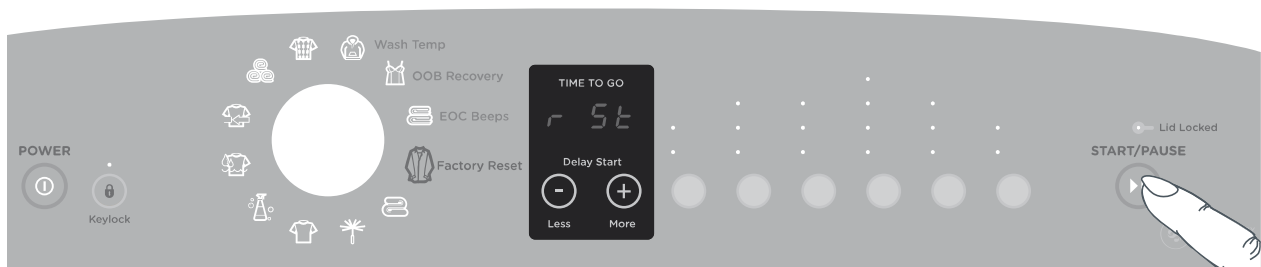
Fig.29 Changing the washer settings back to the factory default
