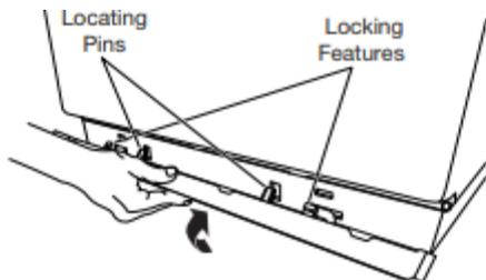
To Install: Place the skirt to bottom of dryer and match the locating pins with the holes. Press the skirt firmly upwards until it snaps into place.
