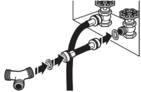
Attach 2 ft. (0.6 m) inlet hose to cold water faucet. Screw on coupling by hand until it is seated on faucet. Then attach "Y" connector to male end of the 2 ft. (0.6 m) inlet hose. Screw on coupling by hand until it is seated on connector.
