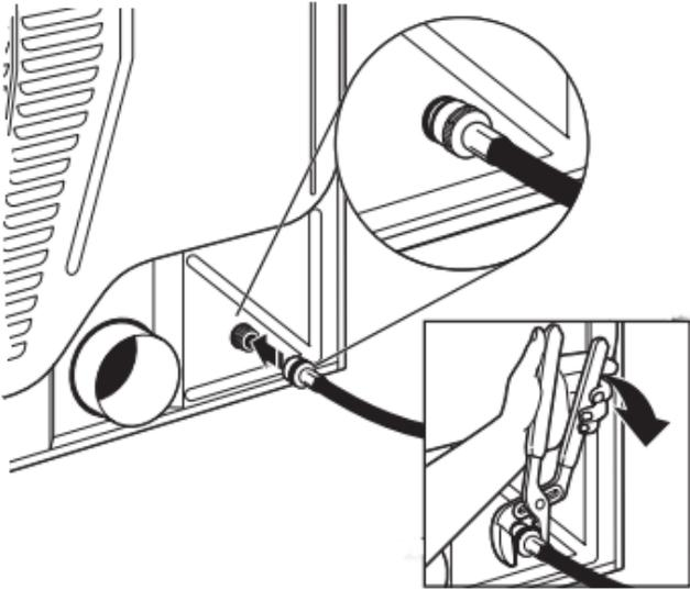
If applicable, remove protective cap from water inlet valve. Attach other end of long hose to fill valve on dryer back panel. Screw on coupling by hand until it is seated on fill valve connector. Using pliers, tighten the couplings an additional two-thirds turn.
