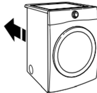
Move dryer to final location. Avoid crushing or kinking vent. After dryer is in place, remove corner posts and cardboard from under dryer.
