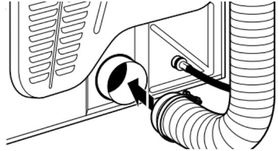
Using a 4" (102 mm) clamp, connect the vent to exhaust outlet in the dryer. If connecting to existing vent, make sure vent is clean. Dryer vent must fit over dryer exhaust outlet and inside exhaust hood. Check that vent is secured to exhaust hood with a 4" (102 mm) clamp.
