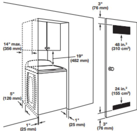
**NOTE:** No other fuel-burning appliance can be installed in the same closet as a dryer.
