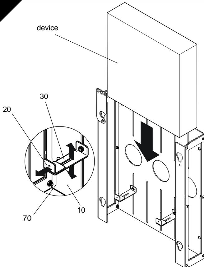
**Adjust Lower device Mounting Brackets**
