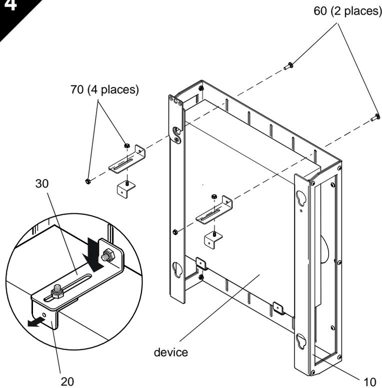
**Install Upper Device Mounting Brackets**
