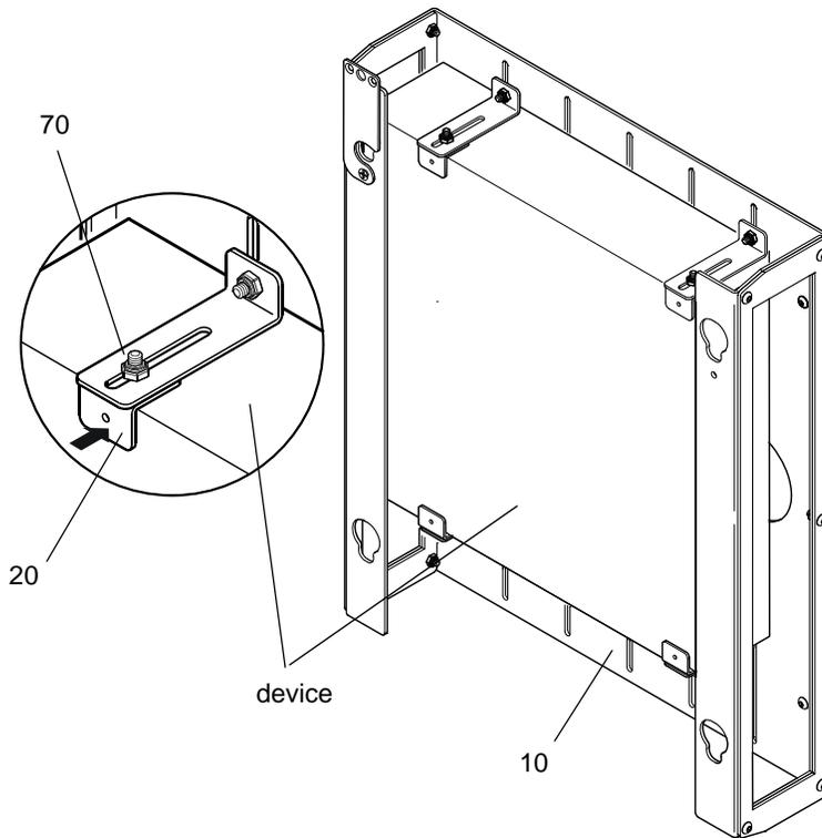
**Adjust Upper Device Mounting Brackets**
