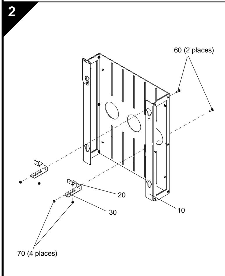
**Install Lower device Mounting Brackets**
