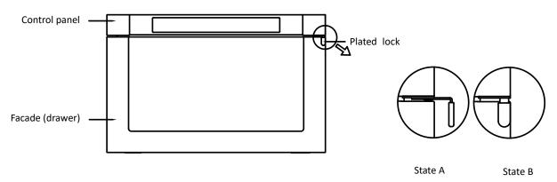
The figure above shows the overall appearance of the drawer type microwave oven and the lock, which are control panel, lock and facade (drawer) from top to bottom.
