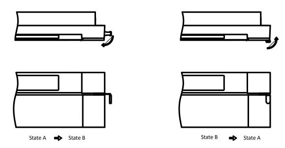
State A -> state B: As shown on the left, rotate the right lock forward 90° to the locking state. State B -> state A: As shown on the right, rotate the right lock 90° to both sides to the locking state.
