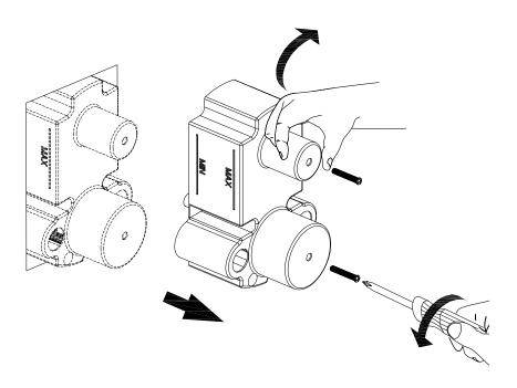
Screw the wall valve body into the system with a screwdriver. Do not overtighten.
