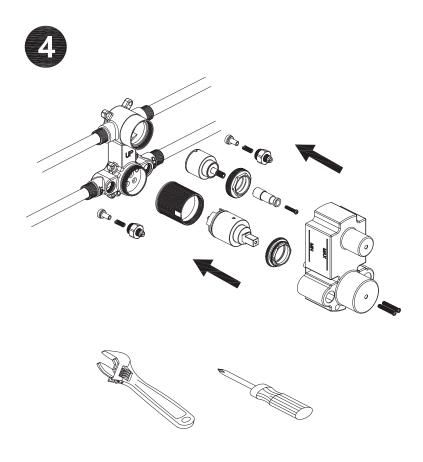
Reinstall the valve components into their original positions.
