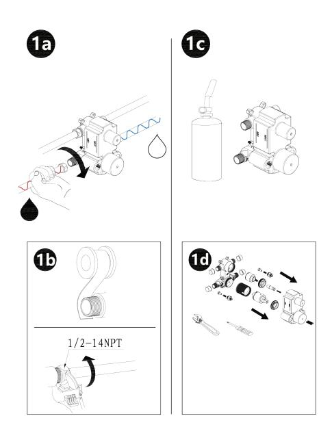
Slide the sleeves onto the pipes and then insert pipes into the wall valve. Tighten the ring around the pipes with the wrench. **NOTE**: If welding is involved, you must remove the internal valve components prior to the welding. Please note the original position of the cartridge.
