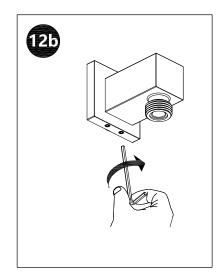
Connect the angle valve to the flange cover and screw together. Secure with plumber's tape to prevent leaks.
