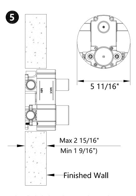
Screw the wall valve body into the system with a screwdriver. Do not overtighten.
