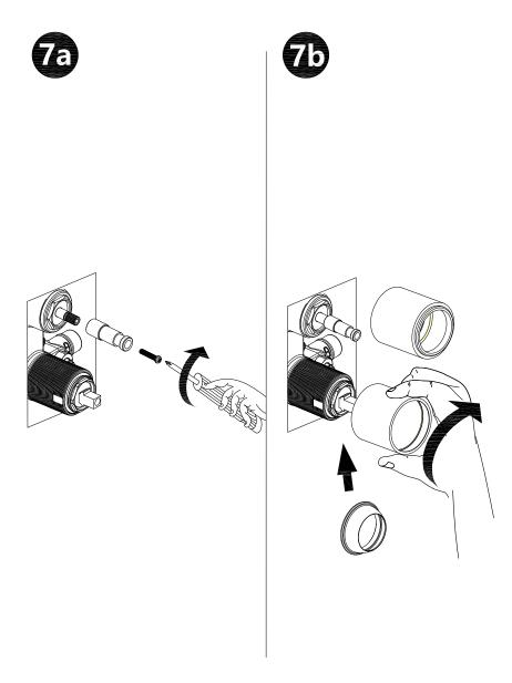
Screw the sleeve and washer into the wall valve body.
