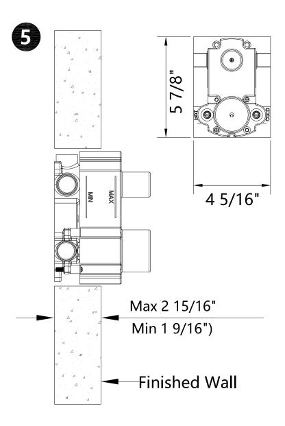
Use this diagram to understand the placement of the wall valve.
