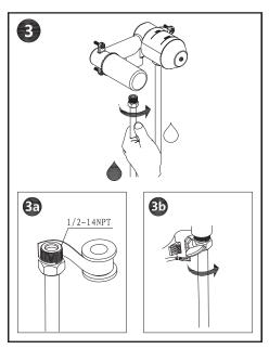
Attach the hose using plumbing tape and a wrench.
