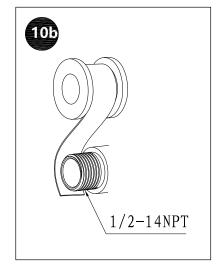
Connect the flange cover to the spout in the wall. Secure with plumber's tape to prevent leaks.
