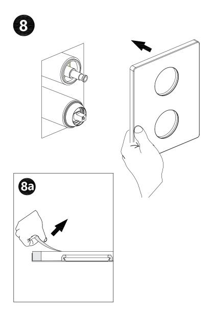
Attach the face plate and remove the plastic.
