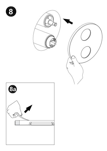
Attach the face plate and remove the plastic.
