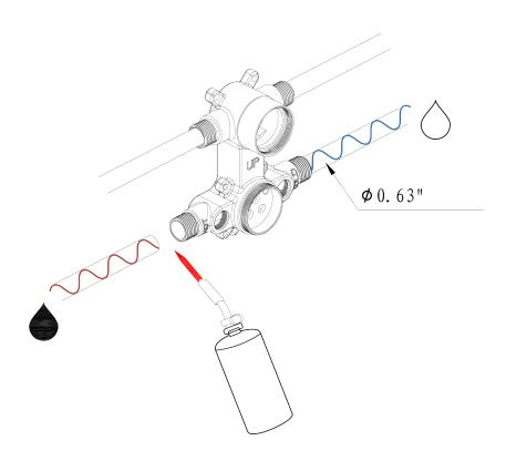
Weld the copper together or use plumber's tape to prevent leaks.
