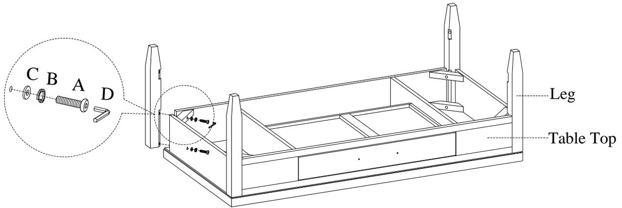
**STEP 2:** Attach the bottom shelf to the legs by using 4 bolts (A), lock washers(B) and flat washers(C). Completely tighten all bolts. Turn the assembled table to the upright position.
