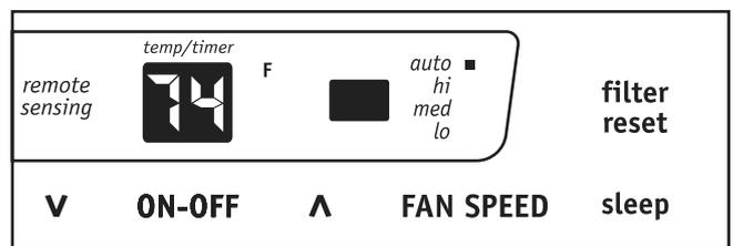
Note: Fan starts at High Speed and adjusts to a slower speeds the room temperature dictates. For example, if the room doesn't get too warm, it will stay at the slowest speed. If the room temperature rises quickly, such as a door being opened, it will automatically go to the highest speed. The fan speeds will re-adjust back to the slowest speed as the room returns to the original set temperature. Press either the fan slower or fan faster button to adjust the fan speed manually.
