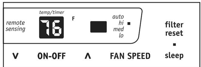
Note: In this mode the selected temperature will increase by 2 °F 30 minutes after the mode is selected. The temperature will then increase by another 2 °F after an additional 30 minutes. This new temperature will be maintained for 7 hours before it returns to the originally selected temperature. This ends the "Sleep" mode and the unit will continue to operate as originally programmed. The "Sleep" mode program can be cancelled at any time during operation by again pressing the "Sleep" button.
