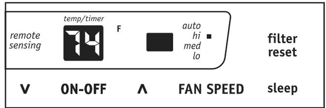
Note: Tap or hold either up ( ^ ) or down ( V ) button until the desired temperature is seen on the display. This temperature will be automatically maintained anywhere between 60 °F (16 °C) and 90 °F (32 °C) . If you want the display to read the actual room temperature. See "To Operate on Fan Only" section on Page 7.
