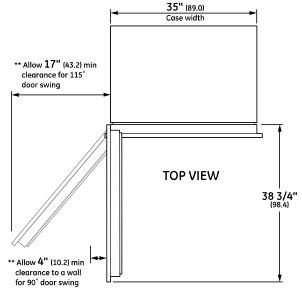
\*\* These freezers are equipped with a 2-position door stop. The factory-set 115° door swing can be adjusted to 90° if clearances to adjacent cabinets or walls is restricted. Allow a 15" minimum clearance to wall for pan removal. If the 90° door stop position is used, pan access is maintained, but pan removal is restricted.
