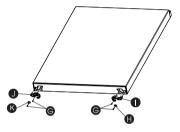
8. Change the screw hole covers and the screws on the middle cover plate from left to right.
