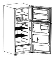
2. With the door closed, remove the upper hinge cover (E) (you can pry it up with a Slotted Screw driver) on the top right side of appliance and remove 3 special flange screws (F) with a Socket Wrench. Keep the upper hinge cover for future reference.
