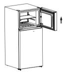
5. Loosen the two screws (G) on the right bottom of the freezer door, then take out the right stopper block (H) and the right door stopper (I). Then install the left stopper block (K) and the left door stopper (J) (provided in the plastic bag).
