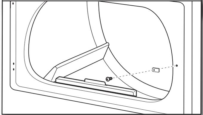
Remove door strike plug. Insert the door strike removed in Step 10 into hole and secure with screw. Insert door strike plug into original door strike hole and secure with screw.
