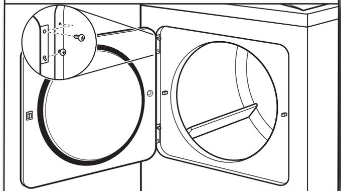
**NOTE:** Two people may be needed to reinstall door. Insert screws into bottom holes on left side of dryer cabinet. Tighten screws halfway. Position door so large end of door hinge slot is over screws. Slide door up so screws are in bottom of slots. Tighten screws. Insert and tighten top screws in hinges.
