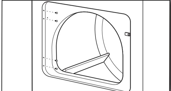
Use a small, flat-blade screwdriver to gently remove 4 hinge hole plugs on left side of dryer cabinet. Transfer plugs into hinge holes on opposite side of dryer cabinet.
