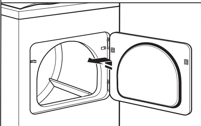
Lift door until top screws in dryer cabinet are in large part of hinge slot. Pull door forward off screws. Set door (handle side up) on top of dryer. Remove top screws from dryer cabinet.
