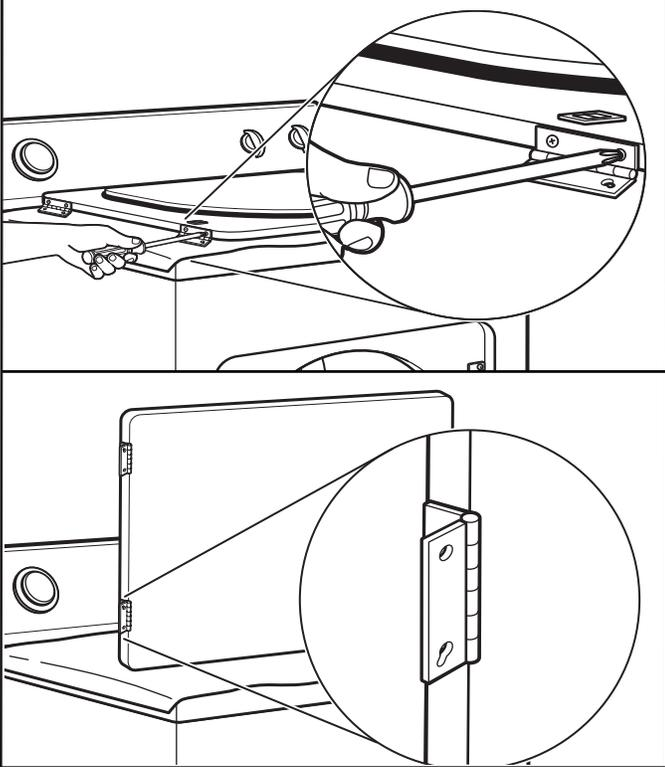
Reattach door hinges to dryer door so that the larger hole is at the bottom of the hinge.
