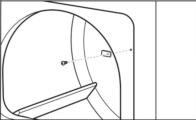
Remove door strike plug. Insert the door strike removed in Step 9 into hole and secure with screw. Insert door strike plug into original door strike hole and secure with screw.
