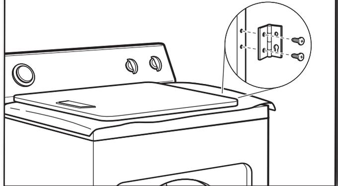
Remove screws attaching hinges to door.
