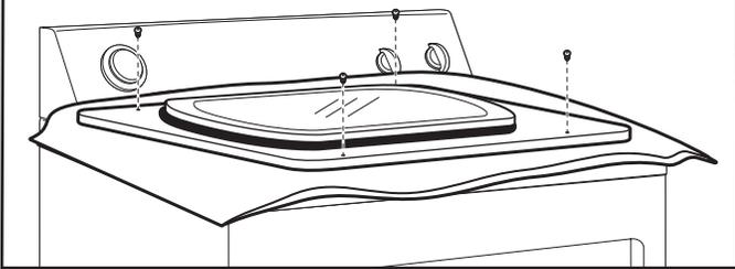
Remove screws at top, bottom, and side of door (4 screws). Keep door screws separate from hinge screws as they are different sizes.
