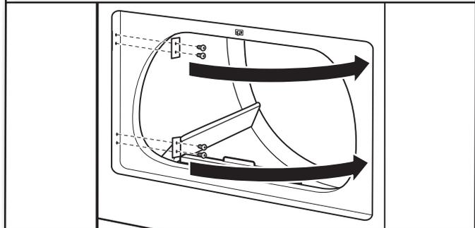
Remove the 4 screws that attach 2 plugs on the left side. Transfer plugs to opposite side using the same 4 screws.
