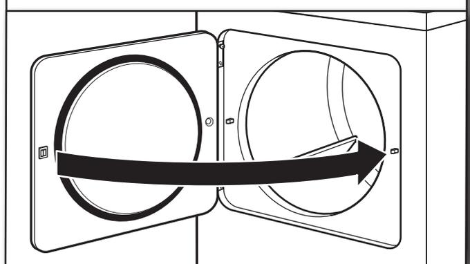
Close door and check that door strike aligns with door catch. If needed, slide door catch left or right within slot to adjust alignment.
