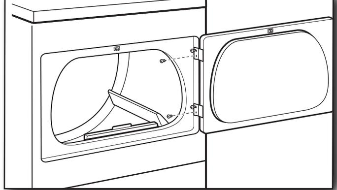
Open dryer door. Remove bottom screws from dryer cabinet side of hinges. Loosen (do not remove) top screws from dryer cabinet side of hinges.
