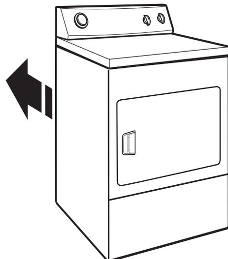
Move dryer to final location. Avoid crushing or kinking vent. After dryer is in place, remove corner posts and cardboard from under the dryer.
