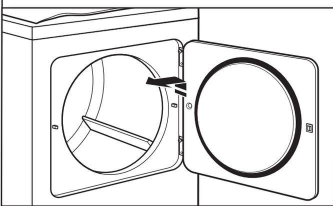
Lift door until top screws in cabinet are in large part of hinge slot. Pull door forward off screws. Set door on top of dryer. Remove top screws from dryer cabinet.
