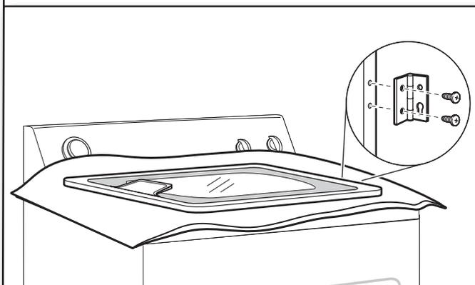
Remove screws attaching hinges to door.
