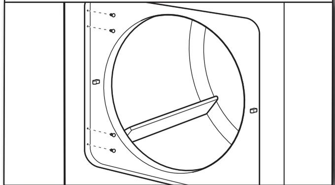
Use a small, flat-blade screwdriver to gently remove 4 hinge hole plugs on left side of dryer cabinet. Insert plugs into hinge holes on opposite side of dryer cabinet.
