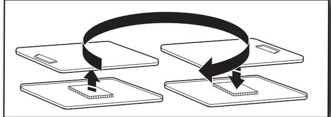
Take outer door and rotate in 180° and set it back down on inner door. Be certain to keep cardboard spacer centered between doors. Reattach outer door panel to inner door panel so handle is on the side where hinges were just removed. Insert 4 door screws.
