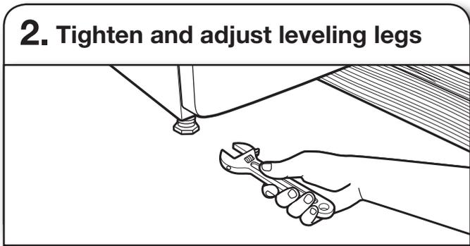
If dryer is not level, prop up using a wood block. Use wrench to adjust legs up or down, and check again for levelness. Once legs are level, make sure all four legs are snug against the floor before tightening them.
