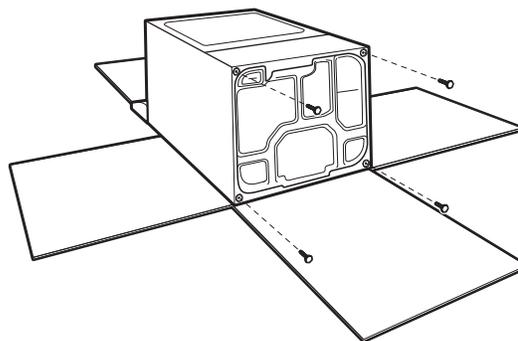
To avoid damaging floor, use a large flat piece of cardboard from dryer carton; place under entire back edge of dryer. Firmly grasp dryer body (not console panel) and gently lay dryer down on cardboard.
