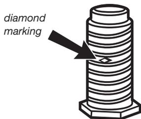
Examine leveling legs and find diamond marking. Screw legs into leg holes by hand. Use a wrench to finish turning legs until diamond marking is no longer visible.
