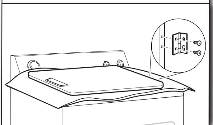
Remove screws attaching hinges to door.
