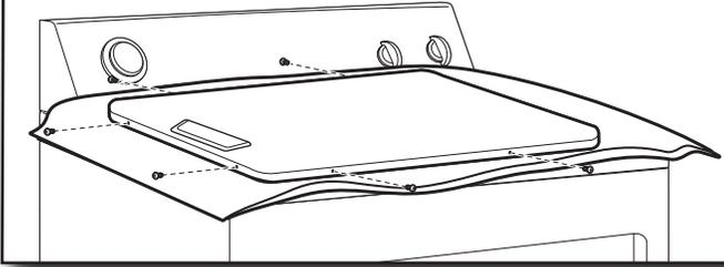
Remove screws at top, bottom, and side of door (6 screws). Keep door screws separate from hinge screws as they are different sizes. Holding door over towel on dryer, grasp sides of outer door and lift to separate it from inner door.
