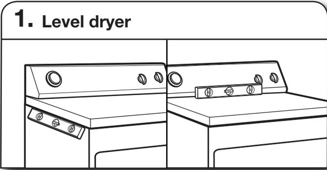
Check levelness of dryer from side to side. Repeat from front to back.
