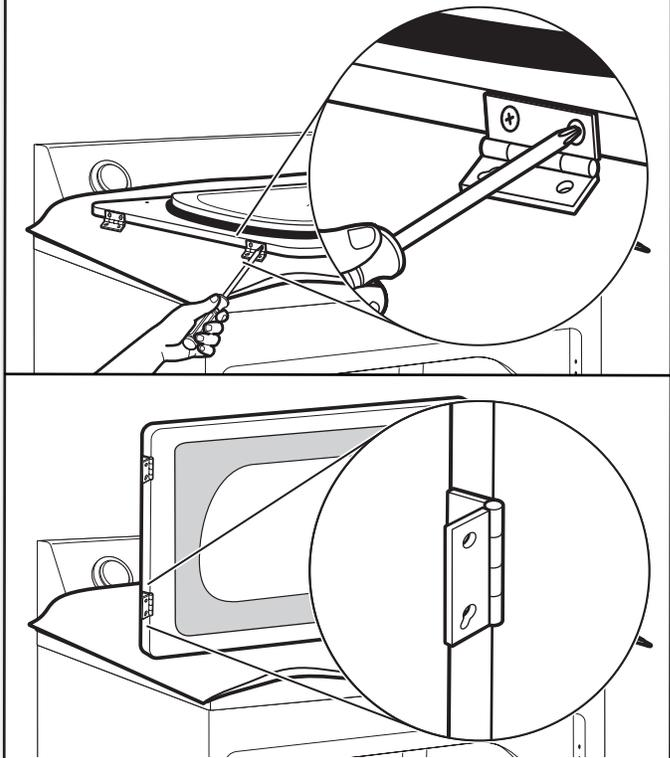
Reattach door hinges to dryer door so that the larger hole is at the bottom of the hinge.
