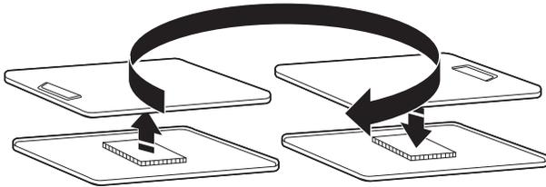
Take outer door and rotate it 180° and set it back down on inner door. Be certain to keep cardboard spacer centered between doors. Reattach outer door panel to inner door panel so handle is on the side where hinges were just removed. Insert 6 door screws.
