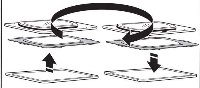
Take outer door and rotate it 180° and set it back down on inner door. Be certain to keep cardboard spacer centered between doors. Reattach outer door panel to inner door panel so handle is on the side where hinges were just removed. Insert 4 door screws.
