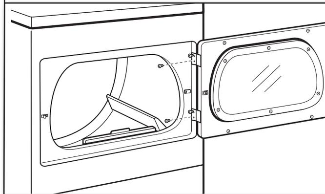
Open dryer door. Remove bottom screws from dryer cabinet side of hinges. Loosen (do not remove) top screws from dryer cabinet side of hinges.
