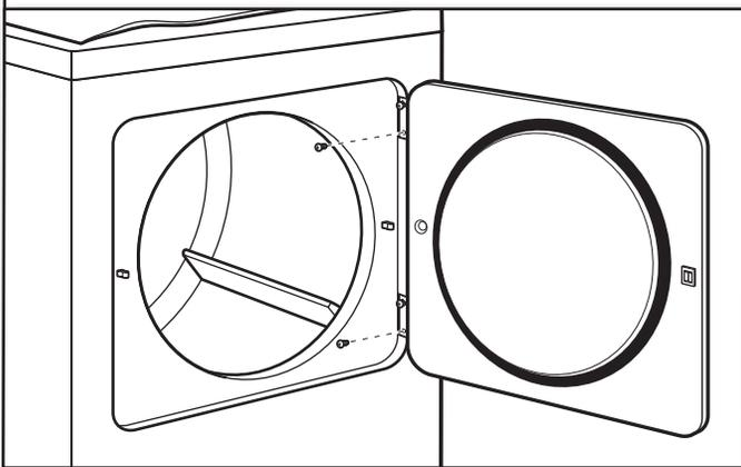
Open dryer door. Remove bottom screws from dryer cabinet side of hinges. Loosen (do not remove) top screws from dryer cabinet side of hinges.
