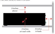
**CAUTION**: Do not block the ventilation holes on the sides and bottom of the AMP-2000.
