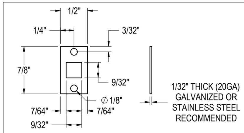
METAL CLIP REQUIRED FOR SNAP IN RETAINER THAT ASSEMBLES GRILL TO THE UNIT. THIS CLIP MUST BE SCREWED TO THE GRILL USING THE FEATURES SHOWN IN DETAIL VIEW "D"
