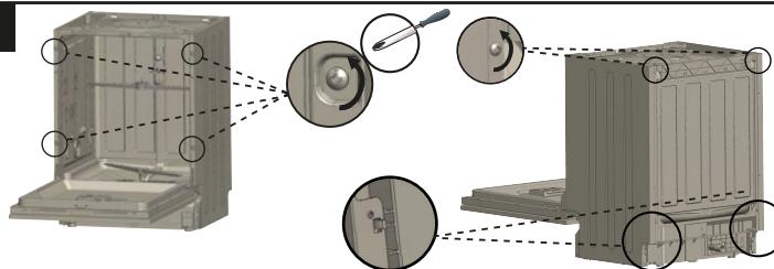
**en** Remove the four screws at front of dishwasher and the two screws at top rear of dishwasher. Unclip the two panel retaining clips at bottom rear of dishwasher.
