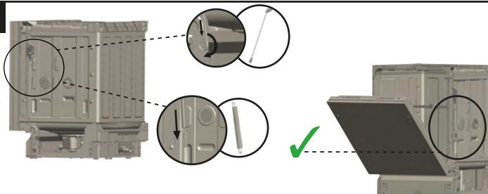
**en** Remove the existing tension spring and install the new tension spring with existing rope.
