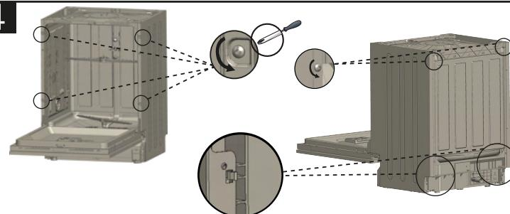
**en** Re-attach the side panels by reclipping lower rear clips and installing the two screws at the rear and the four screws at the front.
