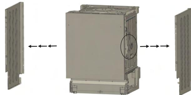
**en** Remove the two side panels to access the tensioning springs.
