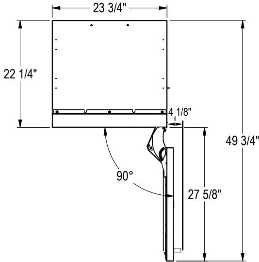
Max clearance required for opened door is 49-3/4" when opened to 90°\* (dimensions shown are without door overlay installed.)
