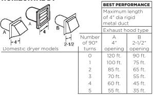
For every extra  $90^{\circ}$  elbow, reduce the allowable vent system length by 10 ft.
