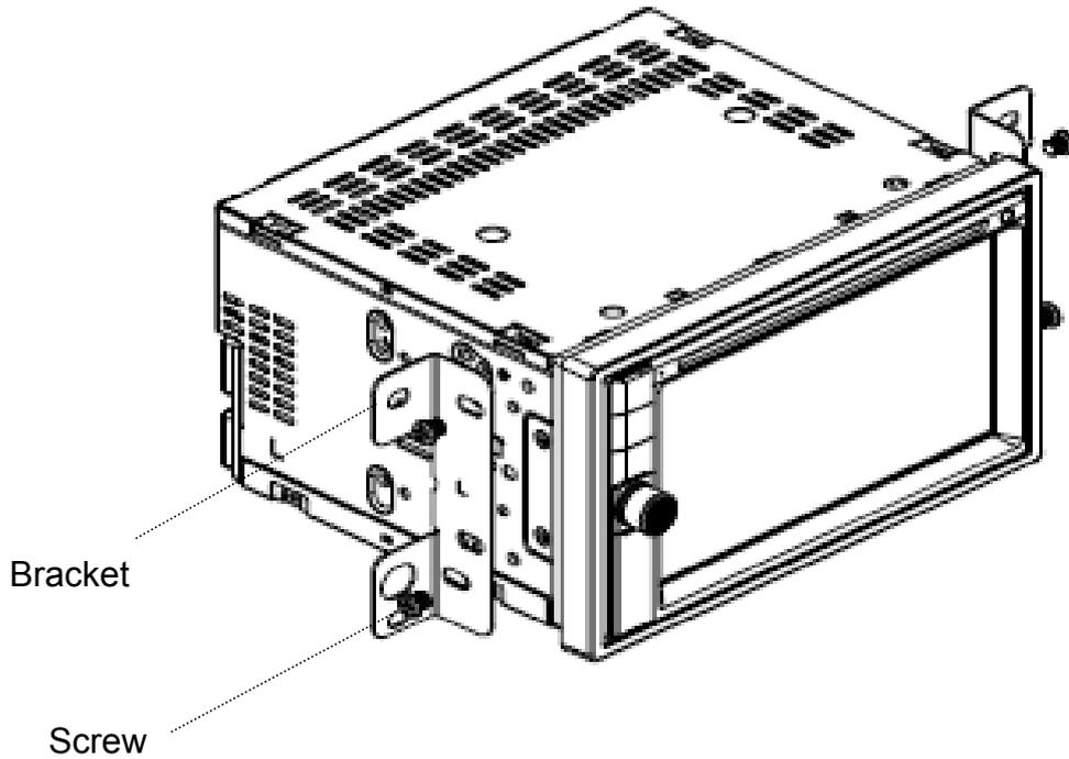
1. Put the 2 brackets to the left and right side of the unit;
