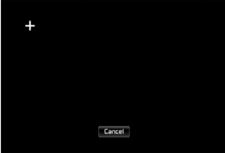
Tap center of the **+** and hold at least 2S, after tap five point, then it will show OK in the picture. and press OK exit calibration mode.
