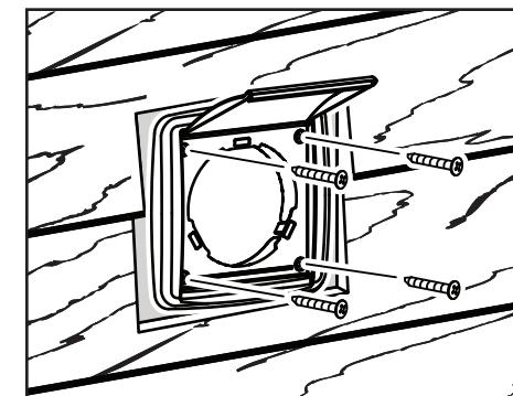
6. Secure vent cover to wall with 4 SCREWS (included). Caulk around vent cover with a quality caulking compound.
