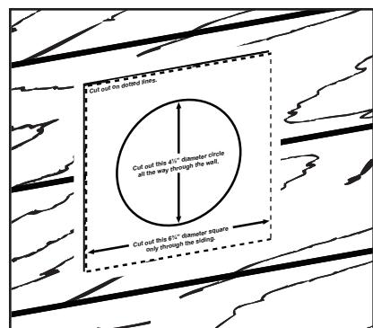
1. Cut out template below and trace outline on wall. Avoid placement where house wiring or plumbing is located.
