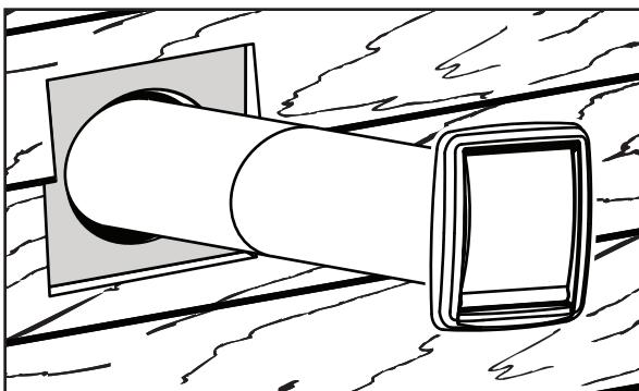
5. Insert duct through hole in wall and fasten duct to metal duct connector. Use duct tape on all connections to make them secure and air-tight.
