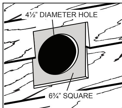
2. Cut 4 1/2" DIAMETER HOLE all the way through the wall. If wall is not flat: Remove any siding or other outer wall covering from inside 6 3/4" SQUARE - to create a flat surface.
