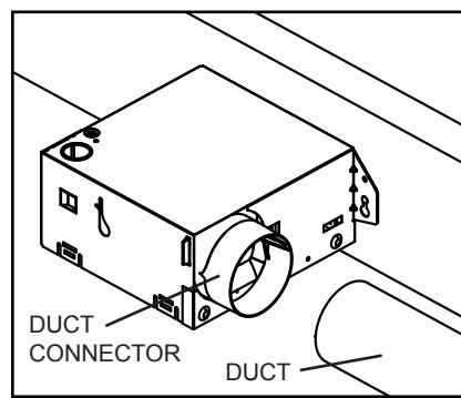
4. Attach DUCT to fan's DUCT CONNECTOR.
