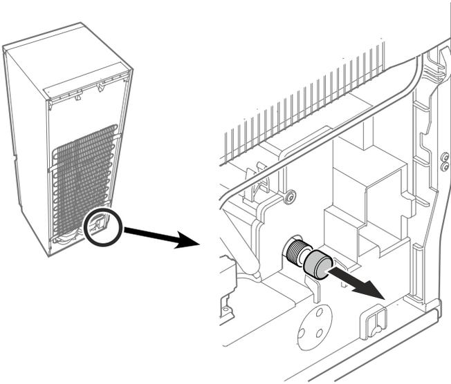
3. Connect the water line to the adapter in the respective configuration, depending on the type of water line used.
