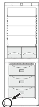
16. Tilt appliance slightly backwards, insert pin and attach using the adjustable foot.
