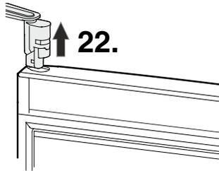
22. Using a screwdriver, push out the hinge and remove it from the door .
