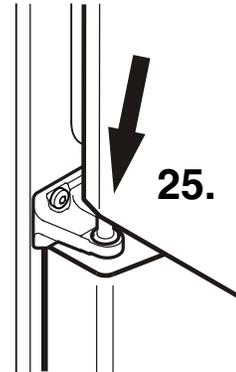
25. Suspend top door on hinge pin. For this, the door must be open at least 90°.
