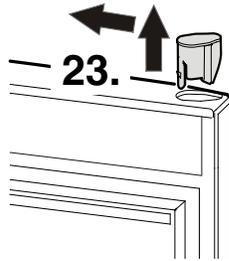
23. Using a screwdriver, push out the plug and transfer it to the opposite side.
