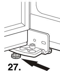
27. Place the appliance in its final position at the place of installation. Extend the adjustable foot at the bottom hinge bracket until it rests on the floor and then make a further 90° turn.
