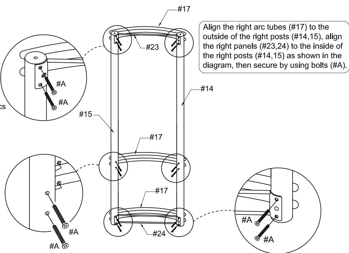
Align the right arc tubes (#17) to the outside of the right posts (#14,15), align the right panels (#23,24) to the inside of the right posts (#14,15) as shown in the diagram, then secure by using bolts (#A).
