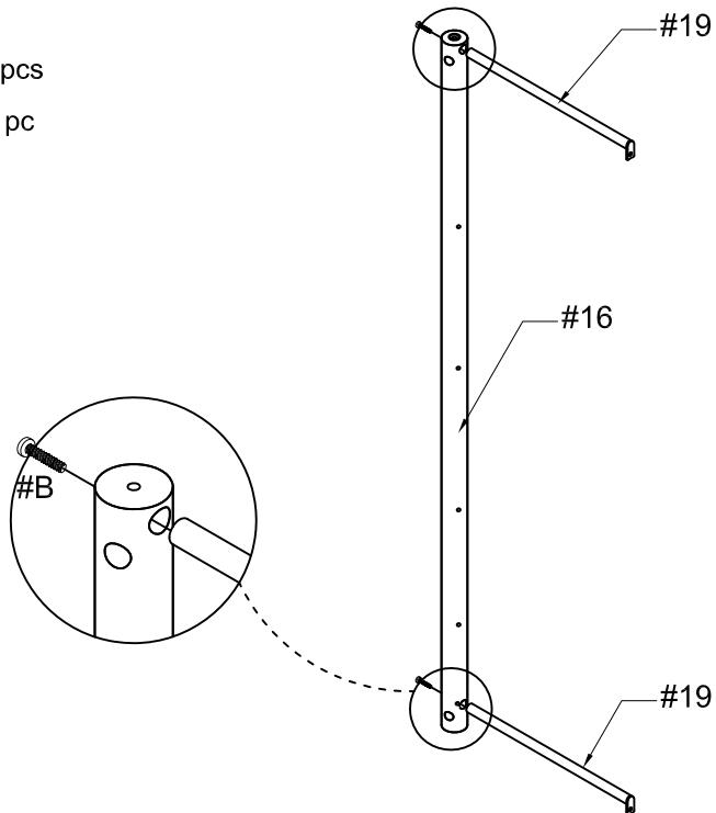
Align the right connection tube 2 (#19) to right post C (#16), then secure by using bolts (#B).
