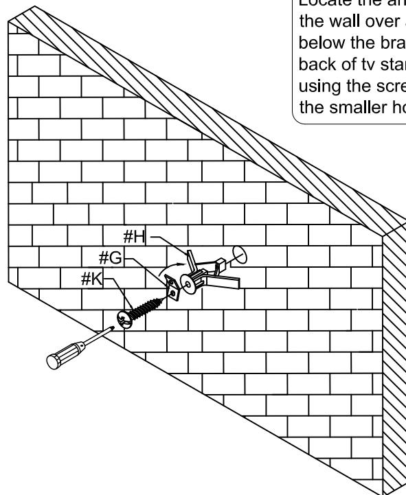
Locate the anchors (H), bracket (#G) on the wall over a wall stud and 2 inches below the bracket (#G) secured to the back of tv stand. Attach the wall stud using the screw (#K) provided, through the smaller hole.
