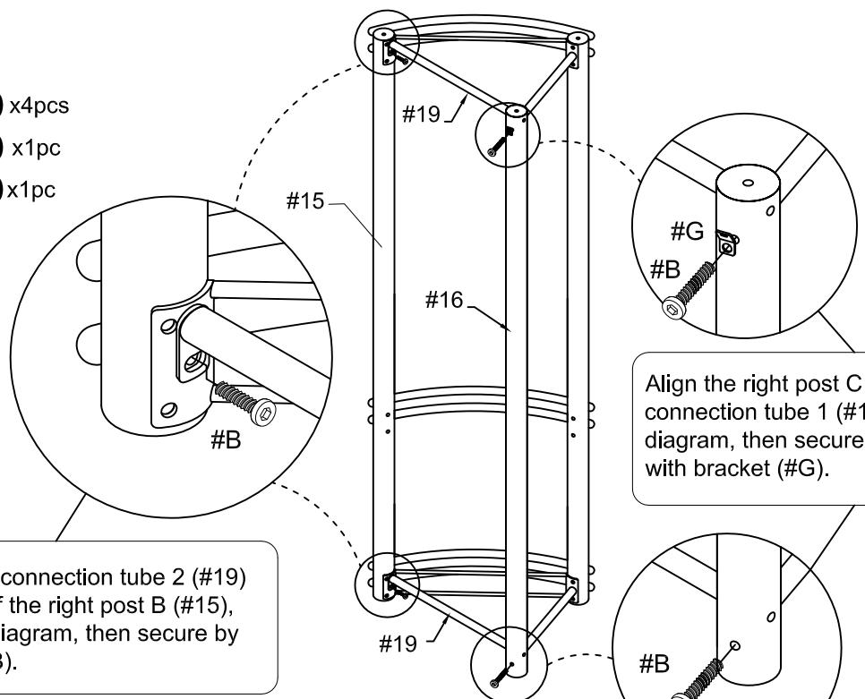
Align the right connection tube 2 (#19) to the inside of the right post B (#15), shown in the diagram, then secure by using bolts (#B).
