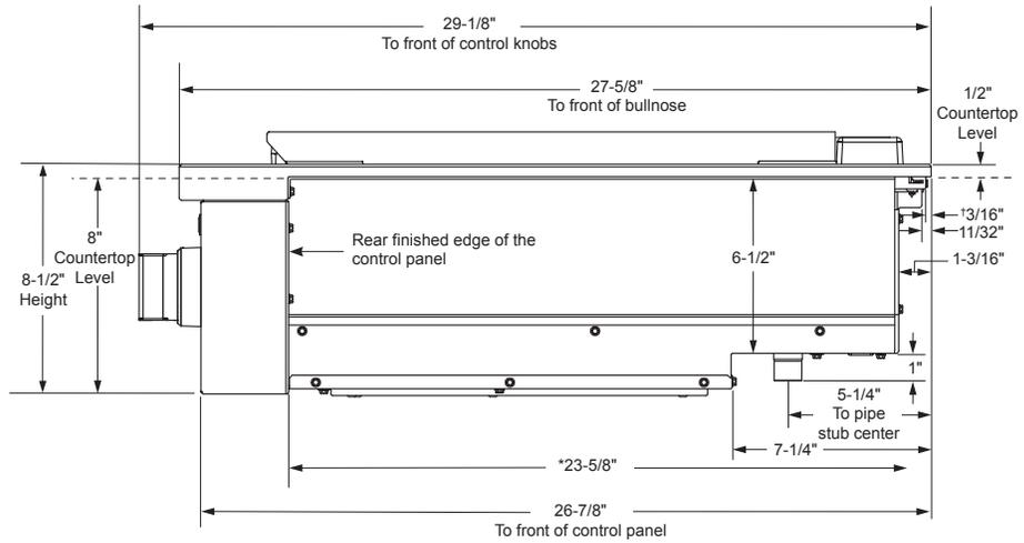
\* Minimum cabinet cutout depth from the back of the rear trim to the back finished edge of the control panel - typically, the minimum cabinet depth (front to back). Maximum cabinet cutout depth is 26" minus the countertop overhang.
