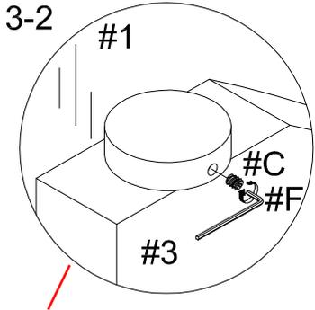
Secure with set screws (#C) to ensure safety of the glass.
