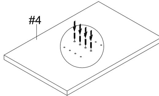
Insert 4 wood dowels (#G) to the holes in the center of the bottom panel (#4).
