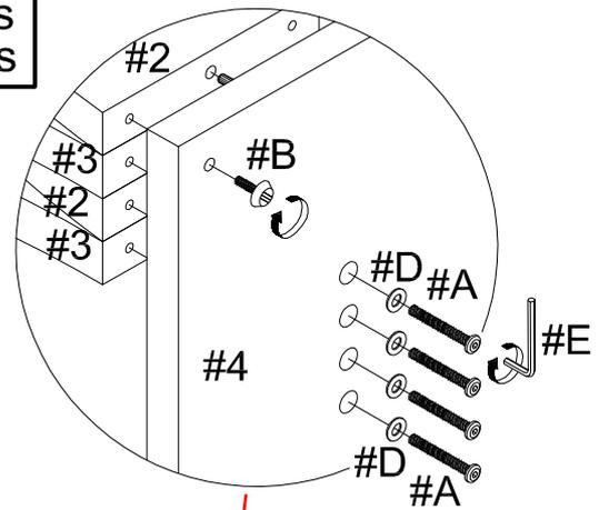
2) Prepare 8 bolts assembly by inserting flat washer (#D) to bolts (#A). Secure panel to legs with bolts (#A). Attach adjustable foot (#B) to the bottom panel (#4) as shown in the picture.
