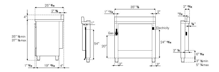
Bertazzoni recommends to operate the appliance after it has been installed in a cabinet. The kitchen cabinets shall be made of materials capable of withstanding temperatures at least 117°F (65°C) above room temperature in order to avoid possible damage to the cabinets during oven usage. For further installation instructions refer to the installation manual
