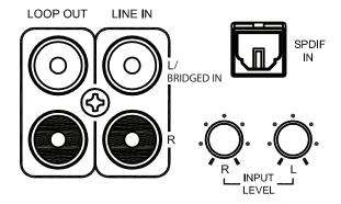
INPUT LEVEL The maximum gain can be set for each channel.
